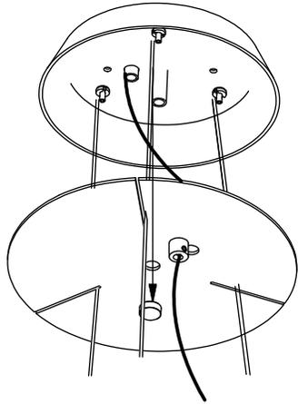
4. (A) CUT THE CABLES TO DESIRED HEIGHT AND PASS THEM THROUGH THE CABLE GRIPPERS
