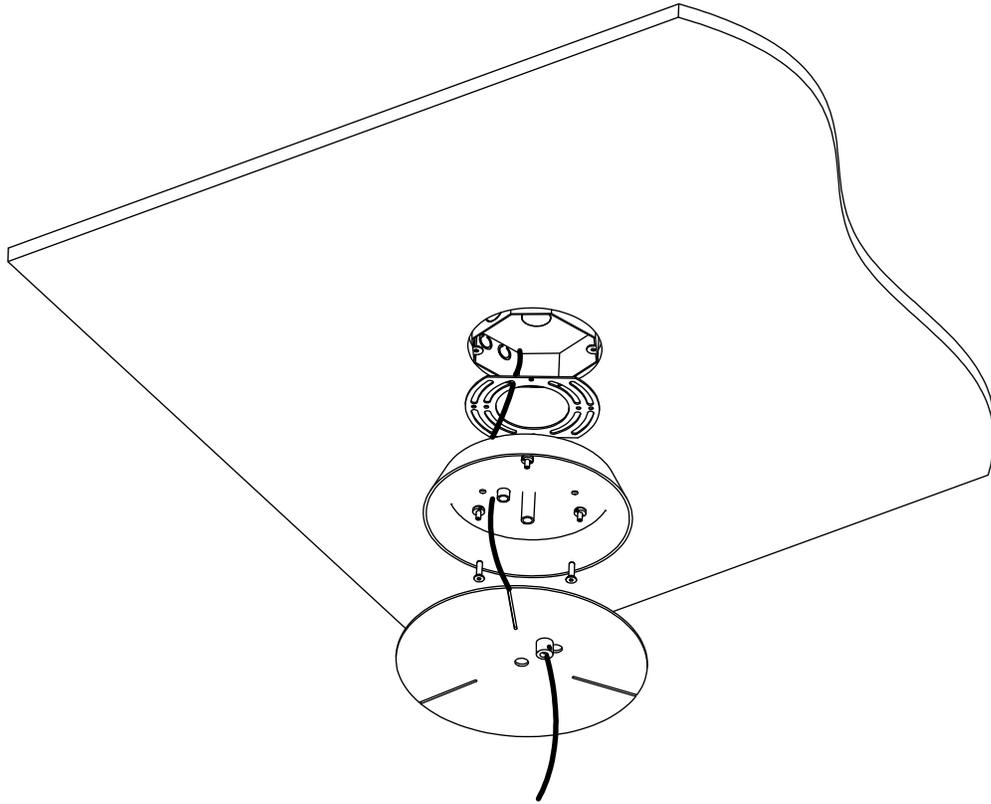
1. (A) INSERT THE CABLE THROUGH BOTH CANOPIES AND MAKE THE ELECTRICAL CONNECTIONS
