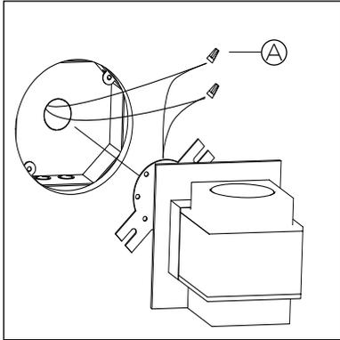
**1 • MAKE ELECTRICAL CONNECTIONS USING APPROPRIATE WIRE NUTS (A) (WIRE NUTS BY OTHERS).**
