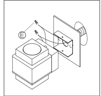
**3 • MAKE ELECTRICAL CONNECTIONS USING APPROPRIATE WIRE NUTS (E) (NOT SUPPLIED).**
