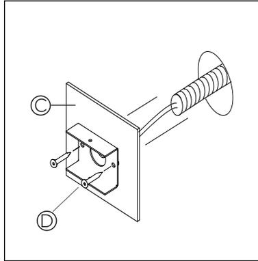
**2 • INSTALL THE FLEXIBLE ARMoured CABLE AND FITTING (NOT SUPPLIED) ONTO THE CANOPY. INSTALL CANOPY ASSEMBLY (C) AGAINST WALL. USE THE RIGHT ANCHORS (D) OR STUDS**
