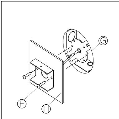
**4 • MAKE SURE MOUNTING SCREWS (F) ARE ALIGNED TO HOUSING'S INNER MOUNTING HOLES (G). INSTALL CANOPY ASSEMBLY (H) AGAINST WALL.**
