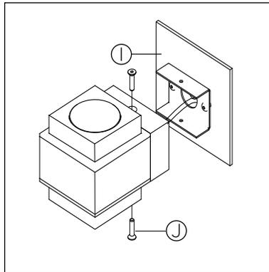
**5 • TUCK IN EXCESS WIRES. FASTEN LUMINAIRE TO CANOPY(I) USING TWO SUPPLIED SCREWS (J). FIRMLY TIGHTEN.**
