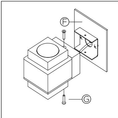
**4 • TUCK IN EXCESS WIRES. FASTEN LUMINAIRE TO CANOPY(F) USING TWO SUPPLIED SCREWS (G). FIRMLY TIGHTEN.**
