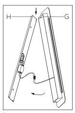
SLIDE CLOSED END OF FIXTURE (G) BEHIND WALL PLATE'S END WEDGE (H). TUCK IN EXCESS WIRE AND CLOSE ASSEMBLY, PUSHING AGAINST WALL PLATE.
