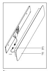
2 • MAKE ELECTRICAL CONNECTION (E) BETWEEN DRIVER AND FIX-TURE ASSEMBLY (F). A CLICKING NOISE CONFIRMS CONNECTION IS PROPERLY LOCKED.
