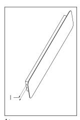
PUSH FIXTURE AGAINST WALL, AND TIGHTEN SET SCREWS (I).
