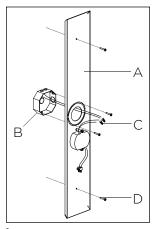
SCREW MOUNTING PLATE (A) TO J-BOX (B) WITH APPROPRIATE HARDWARDE (BY OTHERS). MAKE ELECTRICAL CONNECTIONS USING WIRE NUTS (C). (BY OTH-ERS) INSTALL EXTRA MOUNTING HARDWARE AS NEEDED (D) WITH ANCHORS SUITABLE FOR WALL MATERIAL. (BY OTHERS)
