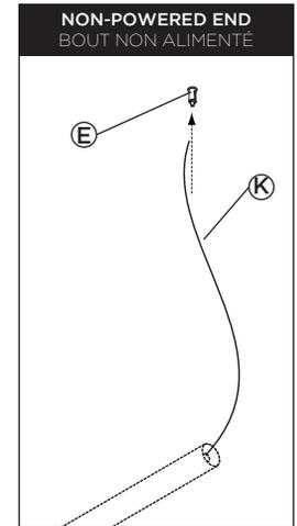
**1 • LOCATE GRIPPERS POSITIONS WITH THE DIMENSION CHART BELOW. PLEASE NOTE FIRST POINT (A) IS NOT AT J-BOX (Q) CENTER (SEE DIMENSION ABOVE). MARK THE POSITIONS FOR GRIPPER POSITION (E).**
