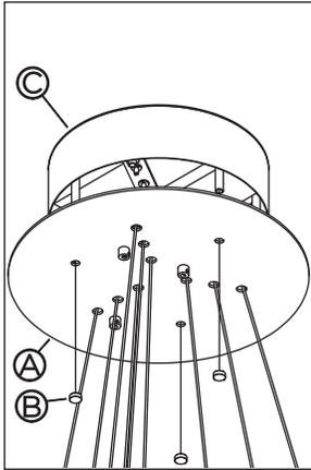
**1 • REMOVE COSMETIC PANEL (A) BY UNSCREWING THE DECORATIVE NUTS (B) AND ACCESS THE INTERIOR OF THE CANOPY (C).**
