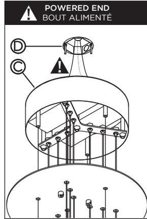
**2 • INSTALL CANOPY (C) TO JUNCTION BOX (D), AND PASS THE CABLES INSIDE THE CANOPY. FASTENERS NOT SUPPLIED.**
