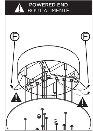
**4 • MAKE ELECTRICAL CONNECTIONS USING APPROPRIATE WIRE NUTS (F) (WIRE NUTS NOT SUPPLIED).**
