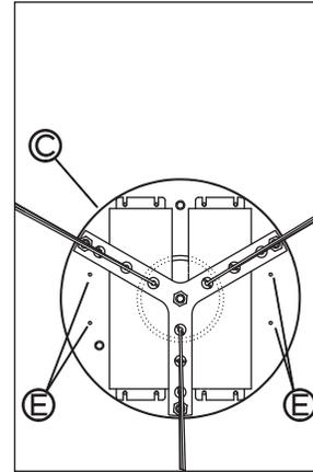
**3 • INSTALL CANOPY (C) TO CEILING THROUGH THE PRE-DRILLED HOLES (E). FASTENERS NOT SUPPLIED.**
