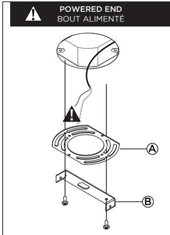
**1 • MOUNT UNIVERSAL PLATE (A) AND CROSS BAR (B) TO J-BOX. (SCREWS NOT PROVIDED).**
