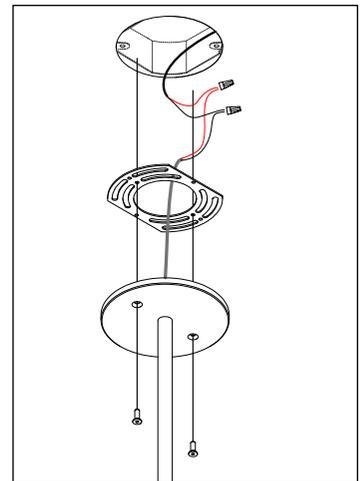
**2 • MAKE THE ELECTRICAL CONNECTIONS IN THE JUNCTION BOX AND INSTALL THE UNIVERSAL PLATE (A). THEN SCREW THE CANOPY IN PLACE (G). FOLLOW STEPS 4 AND 5 TO FINISH INSTALLATION.**
