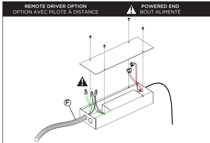
**1 • PULL INSULATED POWER CABLE AND OPEN LID OF HOUSING. INSERT INSULATED CABLE INSIDE HOUSING AND MAKE CONNECTIONS USING APPROPRIATE WIRE NUTS (F). CLOSE THE LID AND PUT THE HOUSING IN THE CEILING. IMPORTANT! USE SCREWS TO FIRMLY FASTEN THE HOUSING IN PLACE.**
