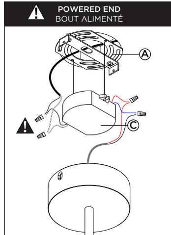
**2 • MAKE THE ELECTRICAL CONNECTIONS AND SCREW THE DRIVER (C) IN PLACE TO THE UNIVERSAL PLATE (A).**
