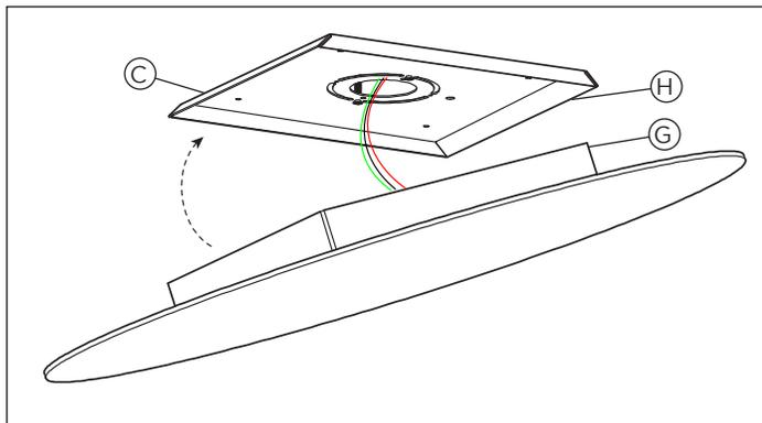
**6 • ALIGN CLOSED END OF FIXTURE (G) TO MOUNTING PLATE'S END EDGE (H). TUCK IN EXCESS WIRE AND CLOSE ASSEMBLY PUSHING AGAINST MOUNTING PLATE (F).**
