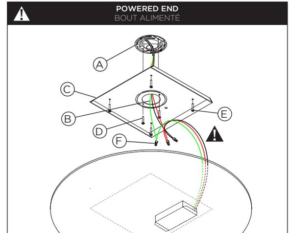
**1 • LOCATE POSITION OF THE FIXTURE. THE J-BOX IS ALIGNED WITH THE CENTER OF THE FIXTURE**
