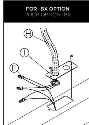
**3 •** INSTALL BX CABLE (H) TO MOUNTING BRACKET (I). MAKE ELECTRICAL CONNECTIONS USING APPROPRIATE WIRE NUTS (F) (NOT SUPPLIED).
