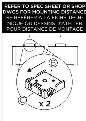
**7 •** MARK MOUNTING POSITIONS AND FASTEN SURFACE BRACKETS (B) TO CEILING, USING APPROPRIATE ANCHORS (NOT SUPPLIED). MAKE SURE BRACKETS ARE ORIENTED TO MATCH MOUNTING FEET (C).
