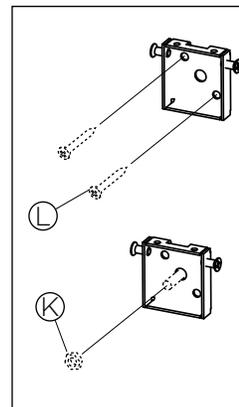
**8 •** DEPENDING ON CEILING SUBSTRATE, SURFACE BRACKETS CAN BE MOUNTED USING #6 SCREWS (L) OR HELD ON 1/4-20 THREADED STUDS USING NUTS (K). (NOT SUPPLIED)
