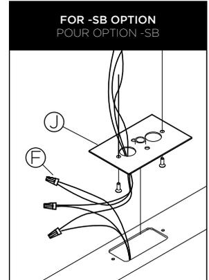
**4 •** INSTALL SWITCH BOX COVER (J) TO SWITCH BOX. MAKE ELECTRICAL CONNECTIONS USING APPROPRIATE WIRE NUTS (F) (NOT SUPPLIED).
