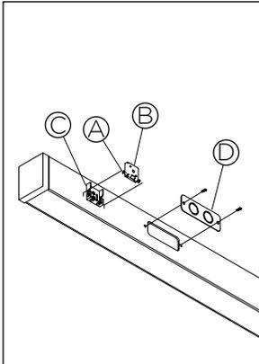
**1 •** LOOSEN SIDE SCREWS (A) ON BOTH ENDS OF FIXTURE TO RELEASE SURFACE BRACKETS (B) FROM MOUNTING FEET (C). DO NOT REMOVE SCREWS. UNSCREW MOUNTING BRACKET (D).
