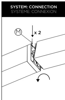
**13 •** TIGHTEN JOINER SET SCREWS (M) FOR ADDED SUPPORT AND ALIGNMENT.
