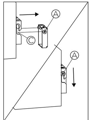
**9 •** ALIGN SURFACE BRACKETS SIDE SCREWS (A) TO CORRESPONDING SLOTS (C) IN FIXTURE MOUNTING FEET AND INSERT. SLIDE FIXTURE IN PLACE, AND TIGHTEN SIDE SCREWS (A) TO LOCK IT.
