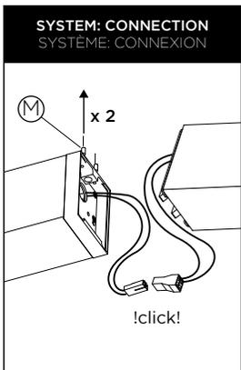
**12 •** LOOSEN JOINER CAP SET SCREWS (M), BUT DO NOT REMOVE. CONNECT NEXT FIXTURE USING PROVIDED QUICK CONNECTORS.
