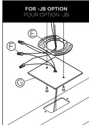
**2 •** INSTALL UNIVERSAL MOUNTING BRACKET (E) TO JUNCTION BOX. MAKE ELECTRICAL CONNECTIONS USING APPROPRIATE WIRE NUTS (F) (NOT SUPPLIED). SCREW CANOPY (G) TO UNIVERSAL MOUNTING BRACKET.
