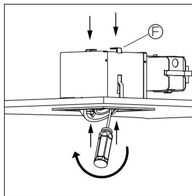
**4 • TIGHTEN MOUNTING SCREWS UNTIL THE TWO CLIPS(F) SECURE THE LUMINAIRE INTO CEILING.**
