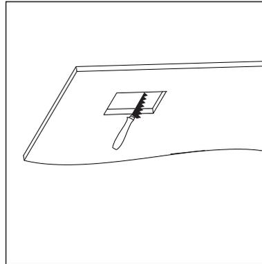
**1 • DISCONNECT POWER BEFORE INSTALLING. DETERMINE INSTALLATION LOCATION AND PRECISELY CUT THE LUMINAIRE'S OPENING.**
