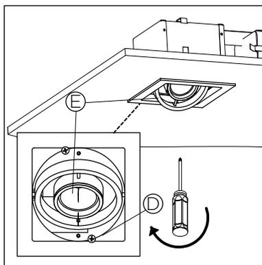
**3 • PIVOT HEAD(E) TO GET ACCESS TO MOUNTING SCREWS(D) INTO FIXTURE.**
