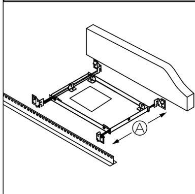
**1 • ADJUST THE WIDTH OF THE HANGER BARS (A) AND SECURE THEM TO JOINTS WITH SCREWS (NOT PROVIDED), OR SUSPENDED CEILING GRID.**
