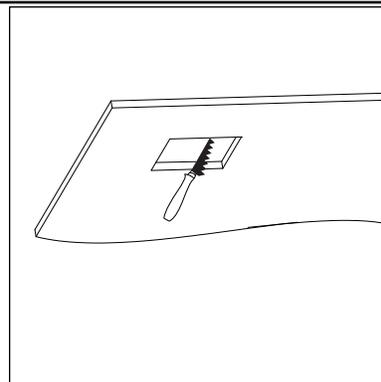
**2 • ONCE DRYWALL IS INSTALLED, PRECISELY CUT THE LUMINAIRE'S OPENING ALIGNED WITH THE HOUSING.**
