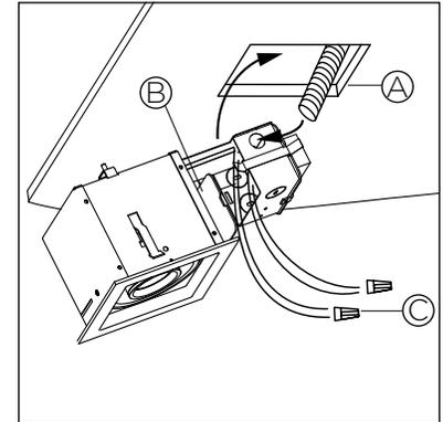
**2 • INSTALL ARMoured CABLE(A) ONTO J-BOX WITH APPROPRIATE HARDWARE (NOT SUPPLIED). REMOVE COVER(B) AND MAKE CONNECTIONS USING APPROPRIATE WIRE NUTS (C) (NOT SUPPLIED). REPLACE COVER AND INSERT FIXTURE INTO CEILING HOLE.**
