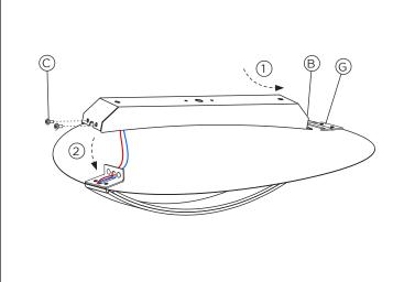
REASSEMBLE FIXTURE BY SLIDING THE EDGE OF CANOPY (B) INTO THE SHADE BRACKET (G) AND ROTATE (1  $\&\,2)$ SCREW SIDE SCREWS (C) TO FIX IN PLACE
