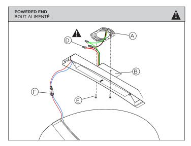
MAKE ELECTRICAL CONNECTIONS WITH WIRE NUTS (D) (NOT SUPPLIED)
