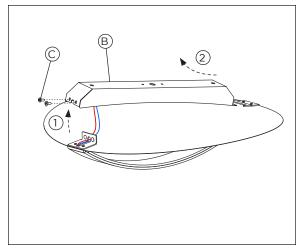
DETACH CANOPY (B) BY UNSCREWING SIDE SCREWS (C) AND BY **ROTATING FIXTURE (1 & 2)**
