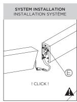
LOOSEN JOINER CAP SCREWS (E), BUT DO NOT REMOVE. CONNECT NEXT FIXTURE USING PROVIDED QUICK CONNECTORS.
