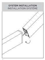
TUCK-IN EXCESS WIRE WHILE INSERTING THE NEXT SECTION'S JOINER CAP HALF INTO THE PREVIOUS.
