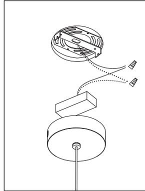
**2 • MAKE ELECTRICAL CONNECTIONS USING APPROPRIATE WIRE NUTS. (WIRE NUTS NOT SUPPLIED).**
