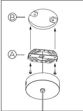
**1 • INSTALL UNIVERSAL MOUNTING BRACKET ASSEMBLY (A) TO JUNCTION BOX (B) USING APPROPRIATE FASTENER (FASTENERS NOT SUPPLIED).**
