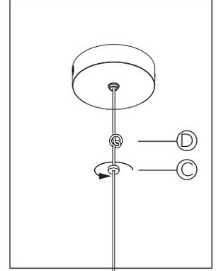
**4 • TO ADJUST ELECTRICAL CABLE LENGTH, RELEASE (C). MAKE A NEW KNOT (D) AT DESIRED LENGTH. SCREW CAP INTO POSITION. (AS PER UL1598)**
