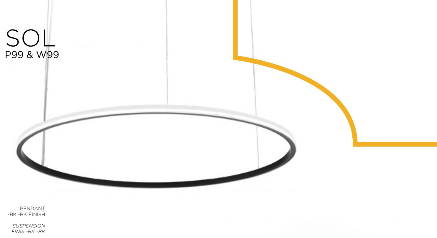
SOL is an elegant and modern thin ring of radiant bright light. Its integral lens, a perfectly diffused satin acrylic piece, is held between fine rims of aluminum. This innovative layered assembly enables mix and match finishes, making a two tone light fixture possible as a standard.
