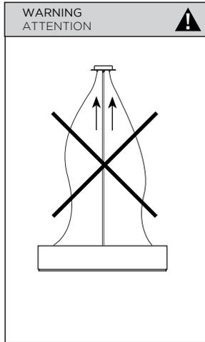
**DO NOT PUT THE WEIGHT OF THE FIXTURE ON THE ELECTRIC CABLE**
