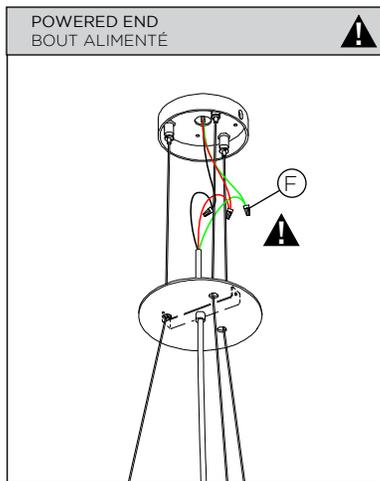
**5 • MAKE ELECTRICAL CONNECTIONS WITH PROPER CONNECTORS (NOT PROVIDED) (F).**
