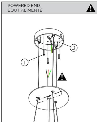
**4 • USE APPROPRIATE SCREWS AND ANCHORS (I) (NOT PROVIDED) TO SECURE CANOPY FRAME (B) TO THE CEILING TAKING INTO ACCOUNT THE WEIGHT OF THE FIXTURE (SEE STEP 1).**
