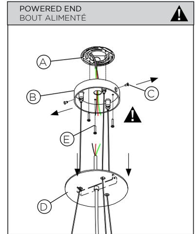
**3 • DETACH CANOPY PLATE (D) BY UNSCREWING THE SIDE SCREWS (C) ON THE CANOPY FRAME (B). PULL PLATE DOWN (D). PULL J-BOX WIRES OUT THROUGH OPENINGS IN CANOPY FRAME (B). FASTEN CANOPY FRAME (B) TO THE UNIVERSAL PLATE (A) USING PROVIDED SCREWS (E).**
