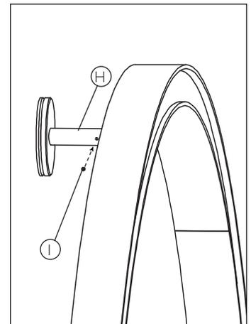
4 • POSITION THE FIXTURE ON THE 3 ANCHORS' TUBES (H) AND FIX THE FIXTURE ON THE ANCHORS BY FASTENING WITH THE 3 INCLUDED SET SCREWS (I).
