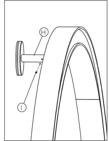
5 • POSITION THE FIXTURE ON THE 3 ANCHORS' TUBES (H) AND FIX THE FIXTURE ON THE ANCHORS BY FASTENING WITH THE 3 INCLUDED SET SCREWS (I).
