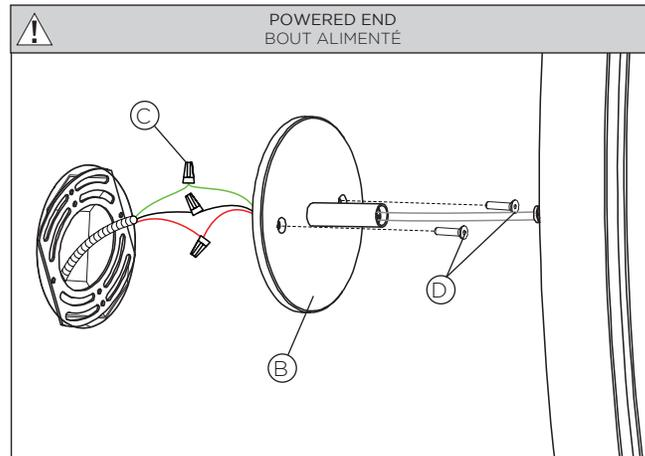
3 • PASS FIXTURE'S CABLES THROUGH CANOPY (B) AND MAKE ELECTRICAL CONNECTIONS WITH PROPER CONNECTORS (C) (NOT PROVIDED). THEN FIX CANOPY (B) TO J-BOX USING PROVIDED SCREWS (D).
