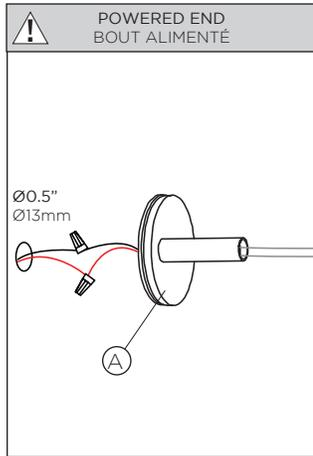
2 • CUT A Ø0.5" HOLE, PASS FIXTURE'S CABLES THROUGH CANOPY (A) AND MAKE ELECTRICAL CONNECTIONS USING APPROPRIATE WIRE NUTS (NOT SUPPLIED). FT4 RATED WIRE SUPPLIED.
