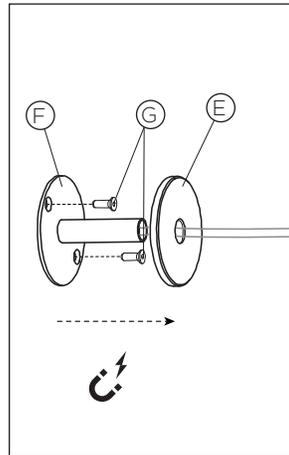
3 • DETACH THE MAGNETIC PLATE (E) OFF THE ANCHORS (F) BY PULLING ON IT. THEN MOUNT ANCHORS (F) TO THE WALL USING PROVIDED SCREWS (G) ACCORDING TO THEIR PREVIOUSLY DETERMINED POSITIONS (SEE CHART 1).
